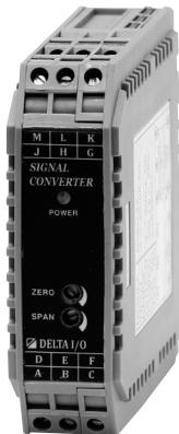
This instrument is a slim type of high accuracy Signal Converter with Power Supply that supplies DC power to 2wire transmitters and derives 4~20mA of DC signal from the DC power as an input, and then outputs the isolated 4~20mA DC signal.
